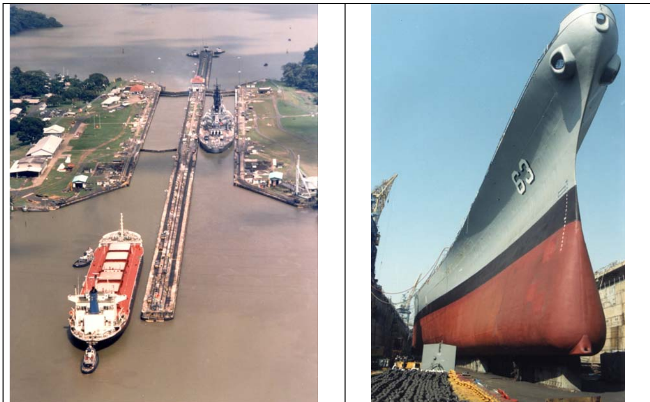
Figure 6 (left) - The width of the IOWA Class battleships was limited by the dimensions of the Panama Canal locks, which were 110 feet wide. The IOWAs employed a beam of 108-1/6 feet. This beam dimension was then multiplied by 7.96 to determine the waterline length of 860 feet. This shows the IOWA transiting the Pedro Miguel Locks on June 6, 1984.
