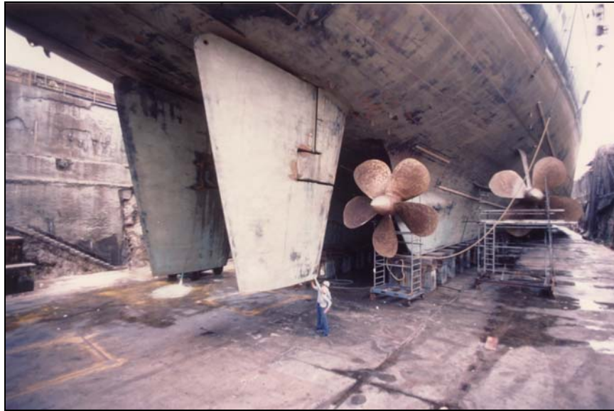
Figure 10 – Propulsion and steering for the IOWA Class battleships included five-bladed inboard screws, 17 feet in diameter, with 4 bladed wing screws 18'-3" in diameter. The design power output was 212,000 shp, with a 20% overload (up to 254,000 shp). During the NEW JERSEY's sea trials in December 1943 the engine room generated 221,000 shp, clocking 31.9 kts with a displacement of 56,928 tons. The IOWA's design speed was about 33.5 kts (38 mph), but a lightly loaded hull (51,000 tons) would have been capable of achieving 35.4 kts (40.25 mph). US Navy photo.
