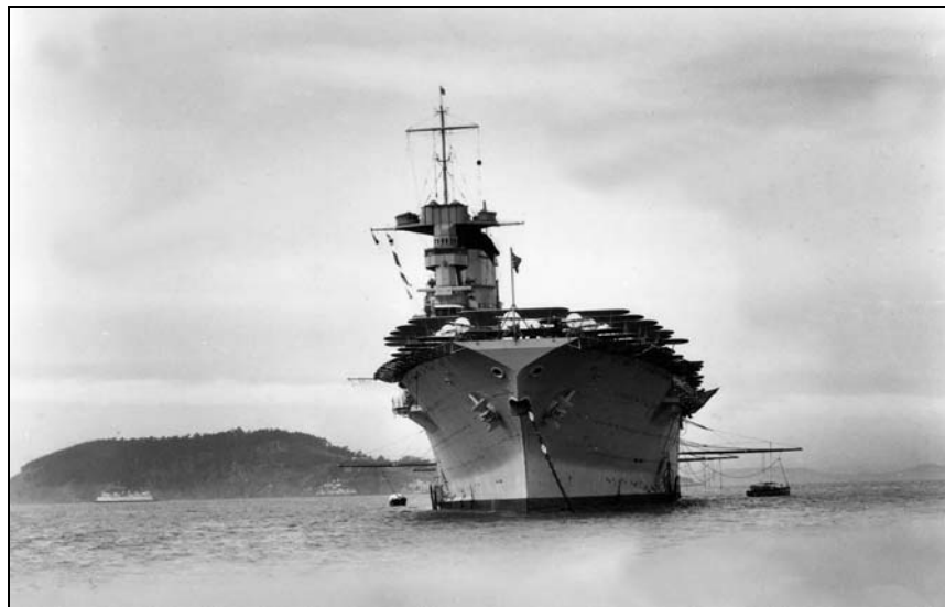
Figure 3 (top) - Bow view of the U.S.S. LEXINGTON (CV-2) at anchor in San Francisco Bay in 1934. The slender sheer of a sleek cruiser hull shows to good effect. The LEXINGTON Class hulls were 26% to 30% complete when original construction was halted in late 1922. This demarcation can be seen as a paint tone change on the hull (photo author's collection).
