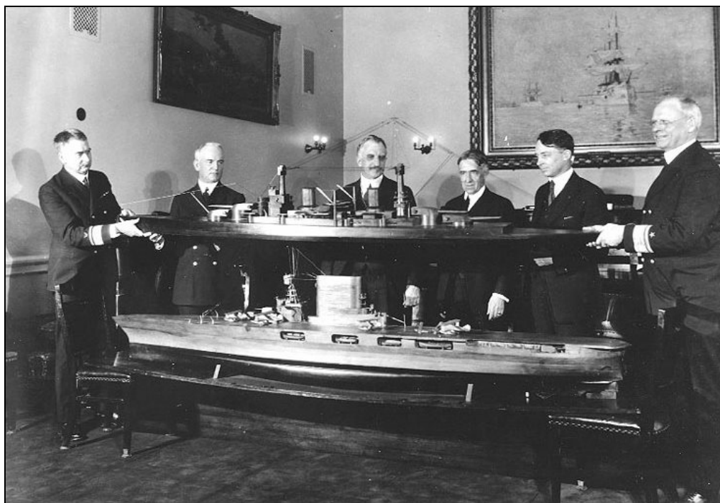
Figure 2 - RADM David W. Taylor (far left), Chief of the Bureau of Construction and Repair, and RADM John K. Robison (far right), Chief of the Bureau of Engineering, hold a model of the LEXINGTON Class battle cruisers under construction in March 1922. In the foreground is a model of an aircraft carrier design converted from the battle cruiser hull, a transformation that was realized for two of the hulls after ratification of the 1922 Washington Naval Treaty. Naval Historical Center photo.
