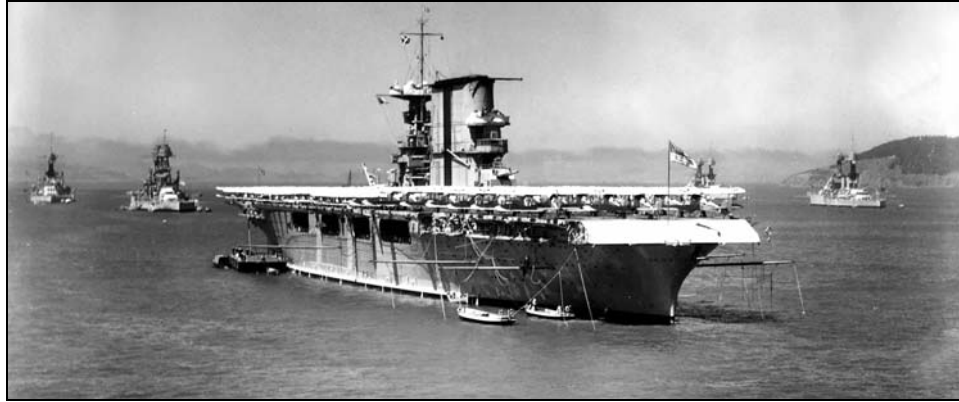
Figure 3 (bottom) - Stern view of the U.S.S. SARATOGA (CV-3) in 1934. The 2-1/2 foot amidships blister and tapered shear of the stern transom are obvious. Note the wide spacing between screws necessitated by the tapered stern section. The single rudder and high slenderness ratio enabled a fast ship, but with poor turning characteristics, which proved troublesome during the Second World War (photo author's collection).
