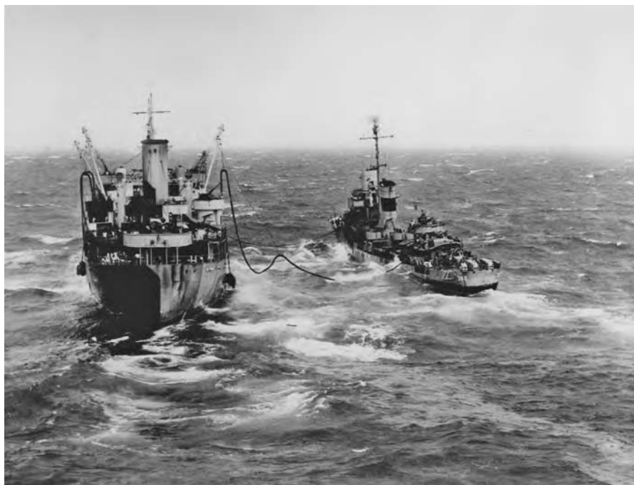
Figure 7-4. A destroyer re-fueling from a fleet oiler. Only the U.S. Navy was capable of alongside fueling; the older refueling method, from a position astern of the delivery ship, was much slower. Underway refueling alongside permitted U.S. Navy ships to remain at sea for extended periods without having to reduce speed to conserve fuel.
