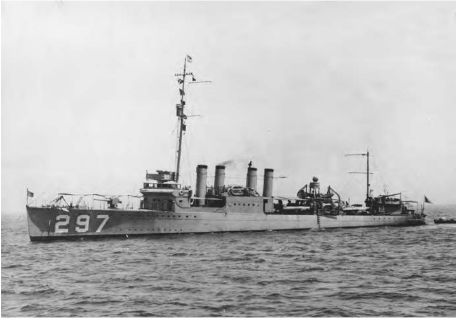
Figure 1–1. The typical World War I type, flush deck, four stack destroyer. These ships also served in World War II and 50 were transferred to the British Navy in 1940.
